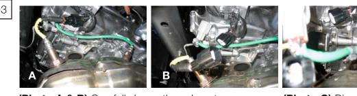
(Photo A & B) Carefully lower the exhaust, but do not remove.
